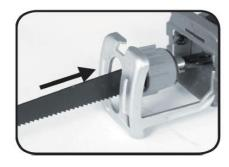
Release the ring on the blade holder and ensure the blade is secure by pulling on the blade
