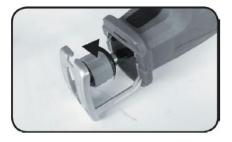
Insert the cutting blade into the slot of the blade holder
