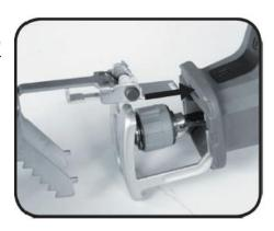
Note: Ensure the clamp is secured by pulling the clamp away from the body.
