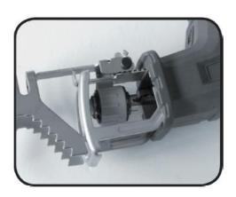
Press and hold the locking button for clamping jaw release into the unlock position.
