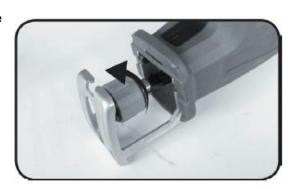
Remove the cutting blade from the blade holder.
