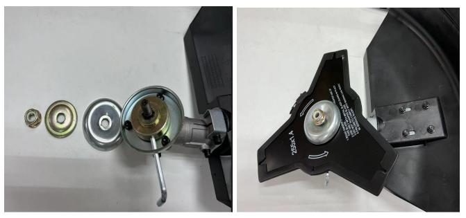
To remove the blade, insert a metal locking tool through the hole on the side of the drive sprocket and on the drive shaft. Loosen the clamp nut, then remove all parts.
