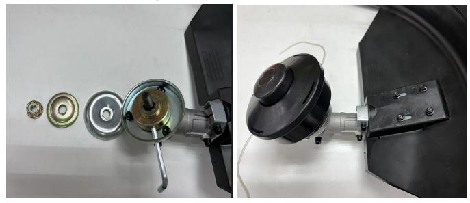
To disassemble the cutting head, insert a metal locking tool through the hole on the side of the drive sprocket and on the drive shaft. Unscrew the cutting head to remove it.
