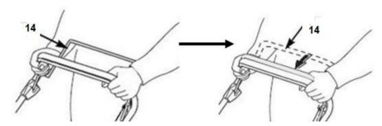
To stop the mower, release the self-propelled lever and then the brake lever.
