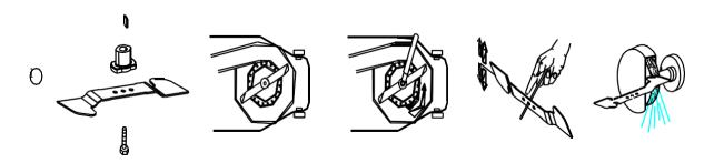
To remove the blade, loosen the screw, check the blade bracket, and replace all parts if they are worn or damaged.
