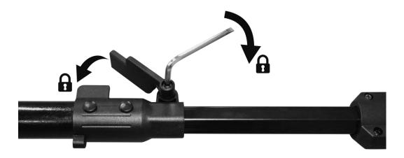
Unscrew, with the provided wrench, the device for the setting of the height of the tool (see above picture). Set the height according the working to do. Put the device in place and screw it firmly.
