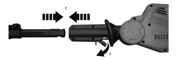
Insert the pole in the tool (1) and press the tab (2). You should hear a click meaning that the pole is locked in the tool.
