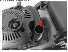
Do not overfill. Wipe off any fuel that has overflowed before starting the engine.
