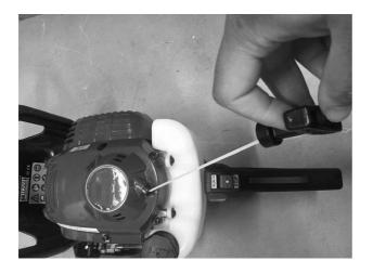
If engine starting is not obtained, put the choke lever on the position **I** and pull again the recoil handle -4 or 5 times and until the tool starts. IłI
