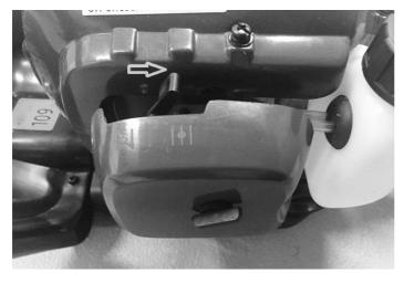
Push and hold throttle trigger lockout (1) and then push the throttle trigger (2). -
