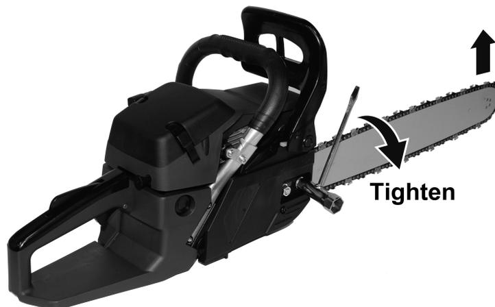
While lifting the chain guide, turn the content screw to apply correct tension to the chain. Then lock the crankcase nuts. Rotate the chain with your hand to check that it is turning without excessive resistance and that it is properly tightened. Repeat the installation if the chain is not tight.
