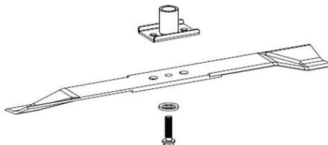
To remove the blade, loosen the screw, check the blade bracket, and replace all parts if they are worn or damaged.
