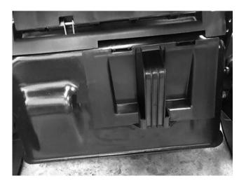
To use the back discharger function, you must open the back flap of the tool. Remove out the mulching adapter on the hole on the back, Release the flap. **NOTE**: do not install the grass catcher when using the mulching adapter. The mulching adapter is not allowed to be fitted when the lateral discharger is used.
