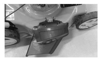
You must fit the mulching adapter in order to use the side ejector. Hook in the side ejector adapter.
