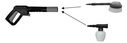
To remove the accessory, push it first and then turn and pull it out from the gun.
