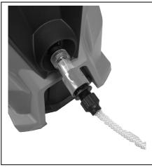
The minimum recommended length for the water supply pipe is 10 meters (but not more than 25 meters) with a diameter of 12.5 mm to avoid back pressure and any potential damage to your appliance. Make sure it can withstand water and a maximum pressure of 10bar (0.1Mpa). If you want to connect your device to other water sources, make sure the maximum water inlet pressure is 10bar (0.1Mpa).
