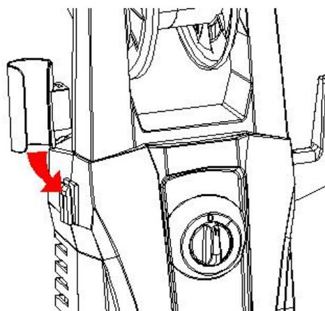
4. Slide the power cord hook into position of unit right.
