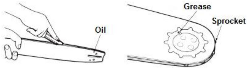
Check: Reverse the bar from time to time to avoid the effects of wear. The bar rail should always be in place. Use a ruler to observe it. If a gap is observed between them, then the rail is normal. Otherwise, the rail is worn out. A bar must be corrected or replaced.
