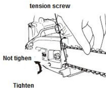
8) Tighten the nuts and check if the chain is rotated correctly and tight.
