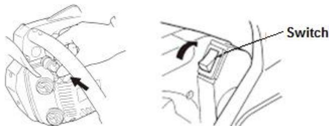
b. Pull the starter button. The starter will close and the throttle will be moved to the starting position
