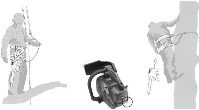
**b. Safe positioning for two-hand operation**
