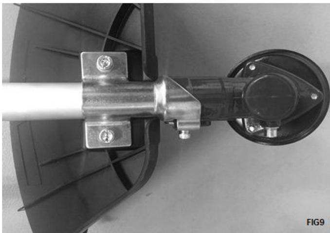
**d) Installation of the nylon cutting head (for grass trimmer operation)**
