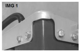
c) Take two M6x16 hex head bolts, two M6 washers and two M6 nuts and mount the guide rail on sides of the table (one horizontal, one vertical). Screw the guide rails. Make sure longer bolts for rails are used.
