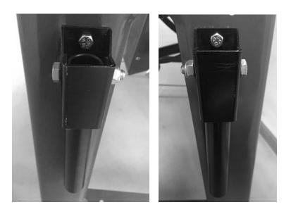
I) Use M6x25 cross groove bolts and M6 nuts, to install the blade protection on the blade.
