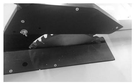
m) Install the rip fence on the guide rail of the table. Check the installation; the device should move freely in the guide rail.
