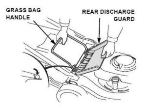
To remove the grass bag, lift the rear discharge guard and remove the grass bag.
