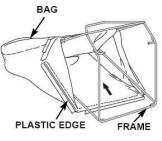
• Insert the frame into the bag, clip the plastic edges of the bag onto the frame.
