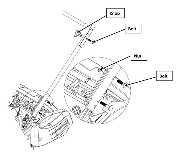
If you want to adjust height of the handle bar, you can choose" L" or "H" two holes in left-right Bracket to fix the handle bar with screws and knobs.
