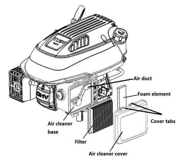
the air filter from the inside. Never try to brush off dirt; brushing will force dirt into the fibers.
