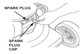
• Remove the spark plug with a spark plug wrench.
