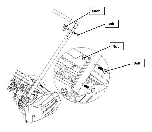
If you want to adjust height of the handle bar, you can choose" L" or "H" two holes in left-right Bracket to fix the handle bar with screws and knobs.
