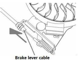
Brake lever cab adjustment
