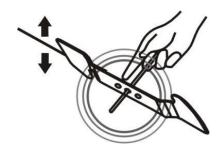
The blade is made of hardened steel. To get a clean job, sharpen the blade frequently, about every 25 hours of use. Make sure the blade is always well balanced.
