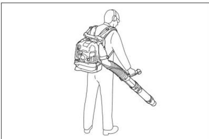
1. While operating the blower, adjust the throttle trigger so that the wind force is appropriate for the work location and conditions.
