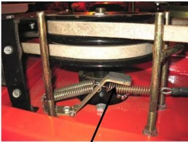
4. The brake pad material should be approximately 1/8-inch thick. Replace the brakes if the material is less than 1/16-inch thick.
