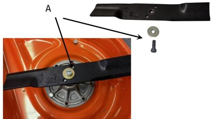
4. To reinstall, fit the blade side holes into the 2 studs to make sure the blade was assembled with right side, and then insert the bolt with lock washer and large flat washer into the spindle.
