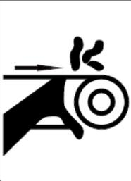
OPEN BELTS & FANS . STOP ENGINE BEFORE REACHING UNDERNEATH .
