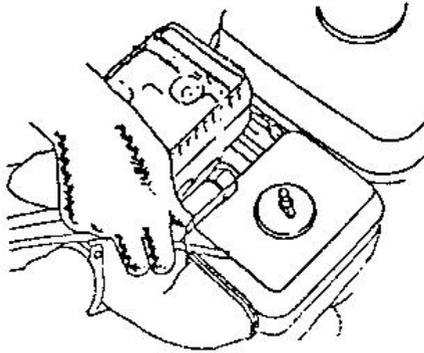
●When mounting a new spark plug, you should screw 1/2 more thread with the wrench after the washer is compressed. If you are mounting an old one, you should only screw 1/8 – 1/4 more thread.
