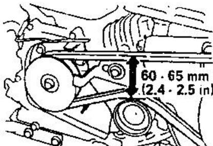
To adjust, loosen the four engine mounting bolts and the engine stay tightening bolt and move the engine forward or reverse to get proper tension of the belt.
