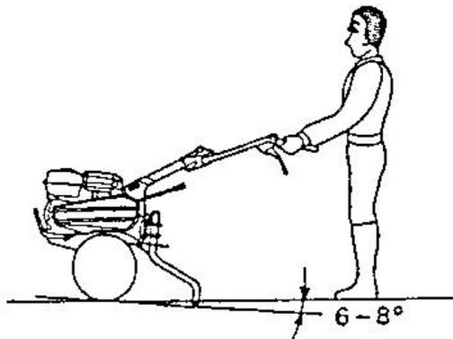
To get the maximum advantage from the tiller, try to hold the machine at the angle shown while you are tilling the ground
