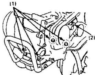
Loosen the attaching bolts of the belt stopper
