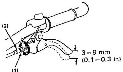
After adjustment tighten the lock nut securely. Then start the engine and check for proper clutch lever operation.
