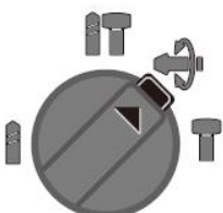
Vario-Lock position for adjustment of the chiseling position
