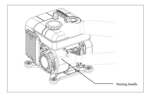
5. After the generator is started, preheat the generator, then slowly turn the throttle arm to the "OPEN" position.
