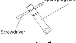
Insert a screwdriver into the spark plug removal tool hole, unscrew the spark plug and remove it
