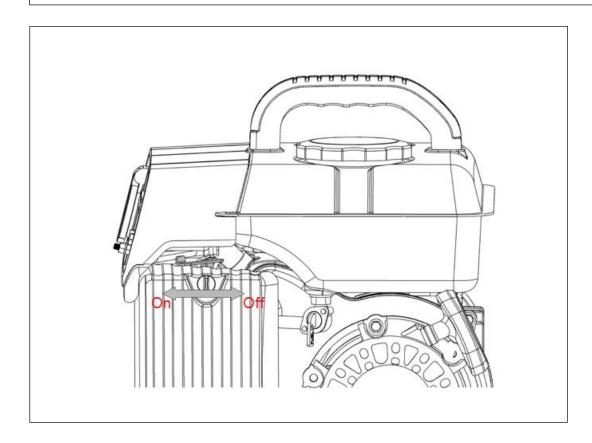
4. Pull the starter handle until you feel resistance, then quickly pull the handle as the direction shown above to start the generator.
