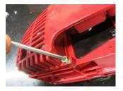
7) Adjust the chain tension by turning the tension screw until the straps touch just the bottom side of the bar.
