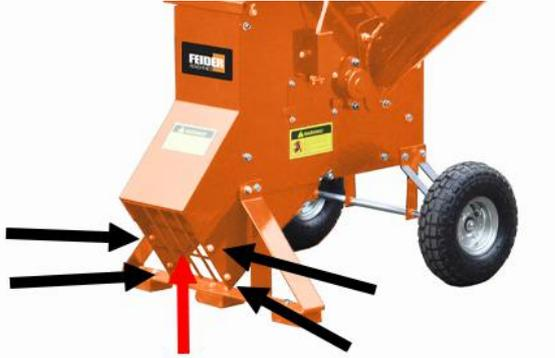
3. Place the handle on the hopper and line up all of the holes. Secure it with flat washer (Ø8, 4pcs), spring washer (Ø8, 4pcs) and bolt (M8x20, 4pcs). (See **Pic.3**)
