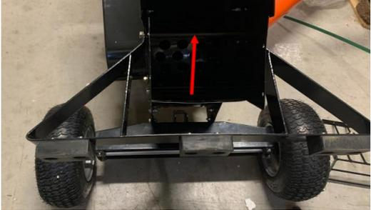
Fit the lower protection grid using the 4 screws and nuts
