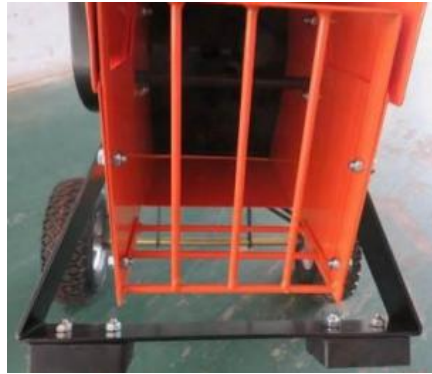
Pic.5 Fence netting installation
