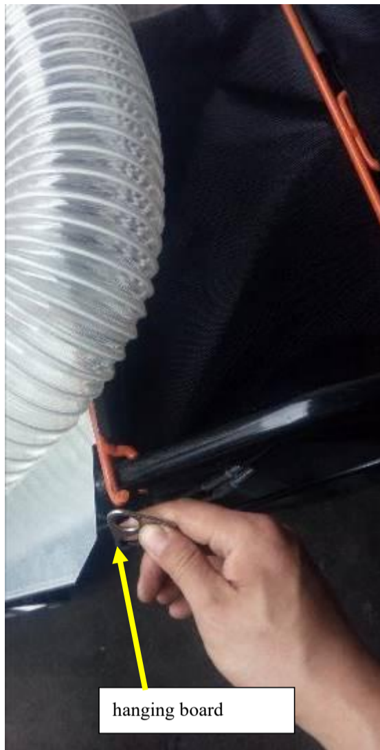
Fig.10-4 Assembly left hanging board
