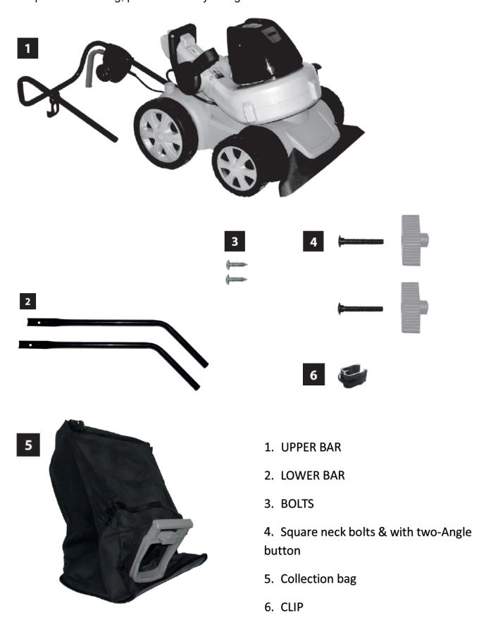
2.2. Insert the lower bar (2) into the holes of deck and lock with the blots(3).
