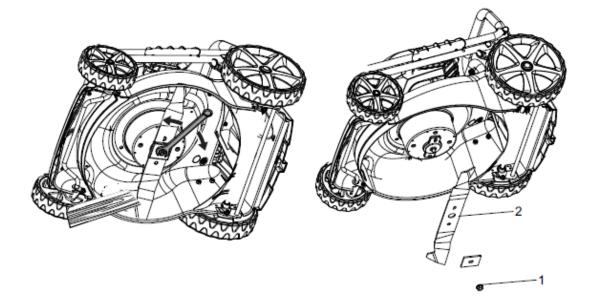
NOTE: Be sure to replace the parts in the exact order in which they were removed. When installing the cutting blade, verify that it is installed with the curved ends pointing toward the mower deck, and not toward the ground.
