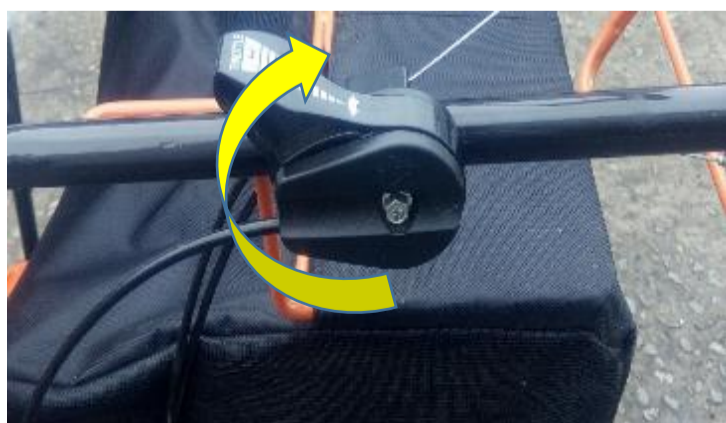
Fig.18-1 Throttle handle- Engine startup state
