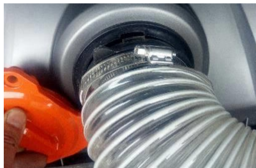
Fig.12-2 Insert hose connector
