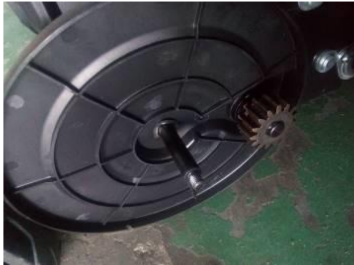
Fig.39-1 Add grease to the gear
