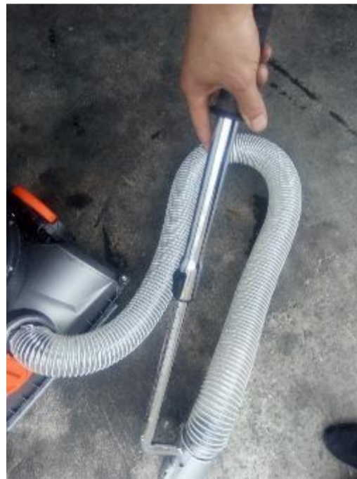
Fig.32-2 Adjust the telescopic height
