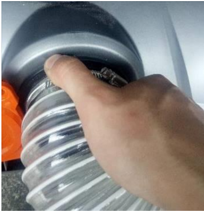
Fig.12-3 Screw the interface
