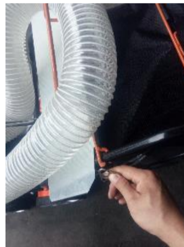
Fig.37-2 Remove the collection bag hanging plate
