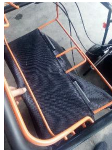
Fig.37-3 Remove the collection bag
