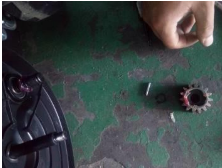
Fig.39-2 Add grease to the output shaft
