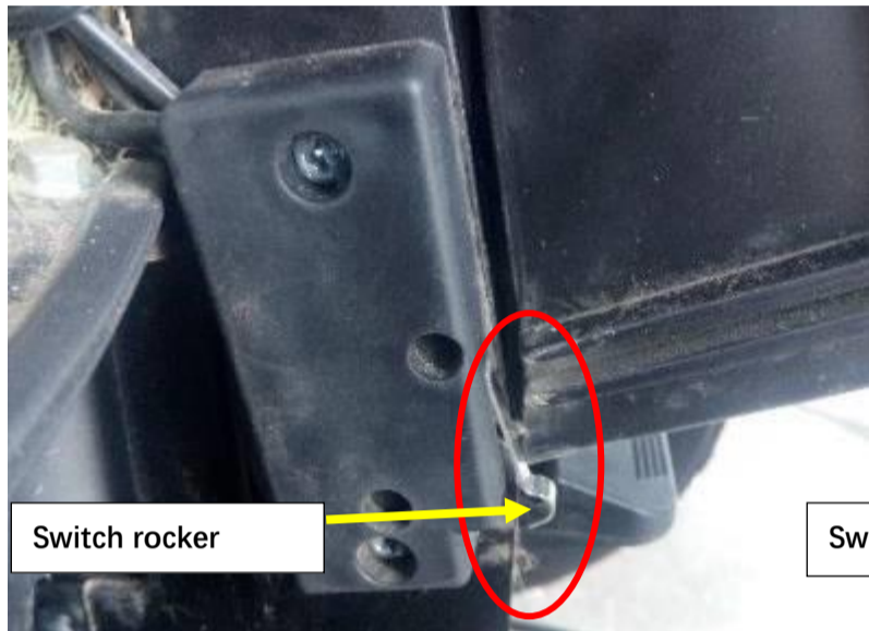
Fig.14-1 Switch rocker- Open state
