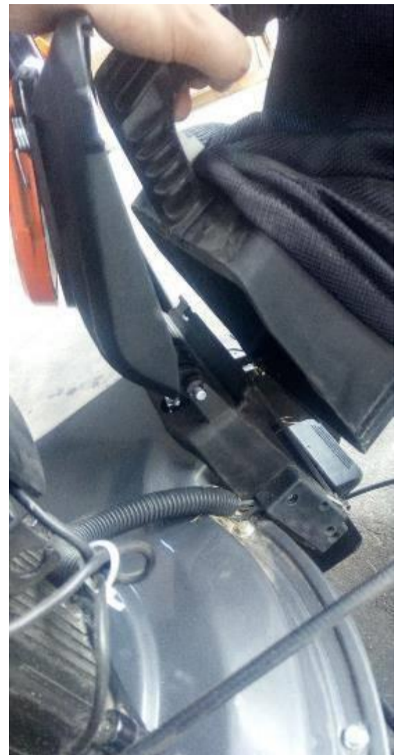
Fig.10-6 Insert back cover bracket
